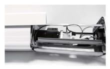
3. Align the camera module to the camera enclosure and slide it back.
