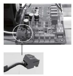
11. Adjust the length of the cable and then tightly screw the cap (see Steps 8 for the picture).
