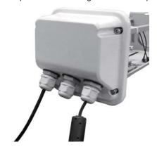
10. Remove the terminal block. Plug black and white wires of the power cable to the terminal block. Reinsert the terminal block onto the camera. The white wire is required to connect to the positive pin (+) on the camera and the black wire to the negative pin (-).
